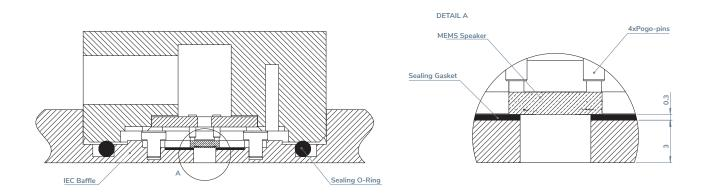
Figure 4: The outlet through the baffle for the speaker has the same shape as the inside of the speaker cover
