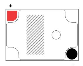
Figure 16: Electrical connections of the speaker back side
