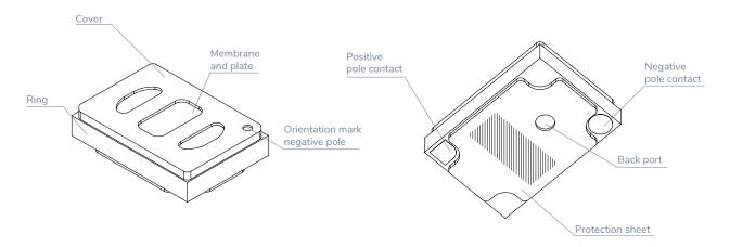
Figure 1: Mechanical drawings: perspective view
