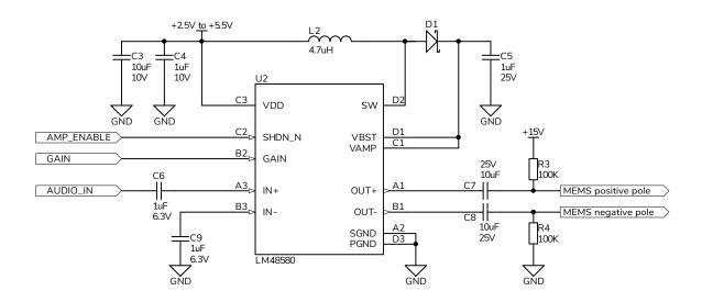
Figure 6: LM48580 amplifier, including required passive components
