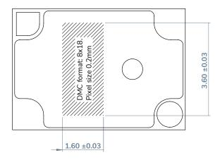
Figure 17: DMC at speaker backside
