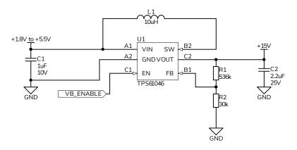
Figure 5: TPS61046 boost converter including required passive components
