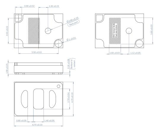
Figure 2: Mechanical drawings: top/down/side view
