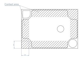
Figure 15: Recommended contact surfaces at the front side (left) and back side (right) of MEMS speaker
