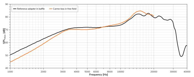
Figure 13: Adap UT-P2023 SPL measurement in the Carme UJ-R1020/UJ-R1030 test box (10 cm) in free field
