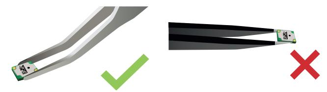
Figure 14: Left: Recommended tweezer type. Right: Not recommended tweezer type
